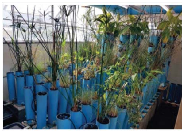
Figure 2-7: Plant biofilter experiment, Stellenbosch University (2018)
