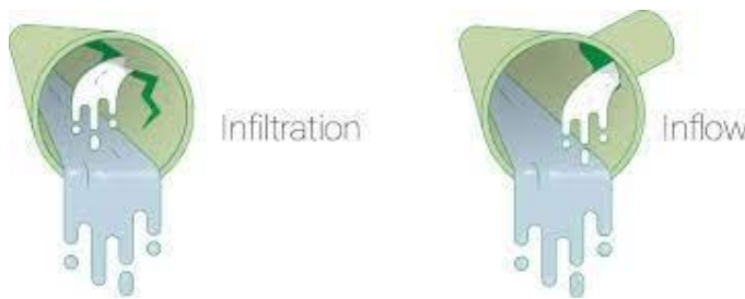
Figure 20. Infiltration and Inflow [25].
