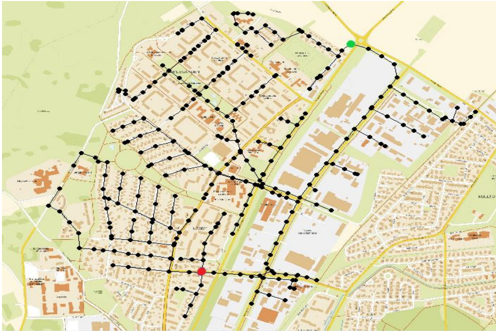
Figure 3. Map of Näsby sewage network superimposed over a map of Näsby, the red mark is the location of the larger pipe and the green mark is the location of the smaller pipe [21].
