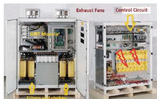
Figure 70: Central inverter internal structure
