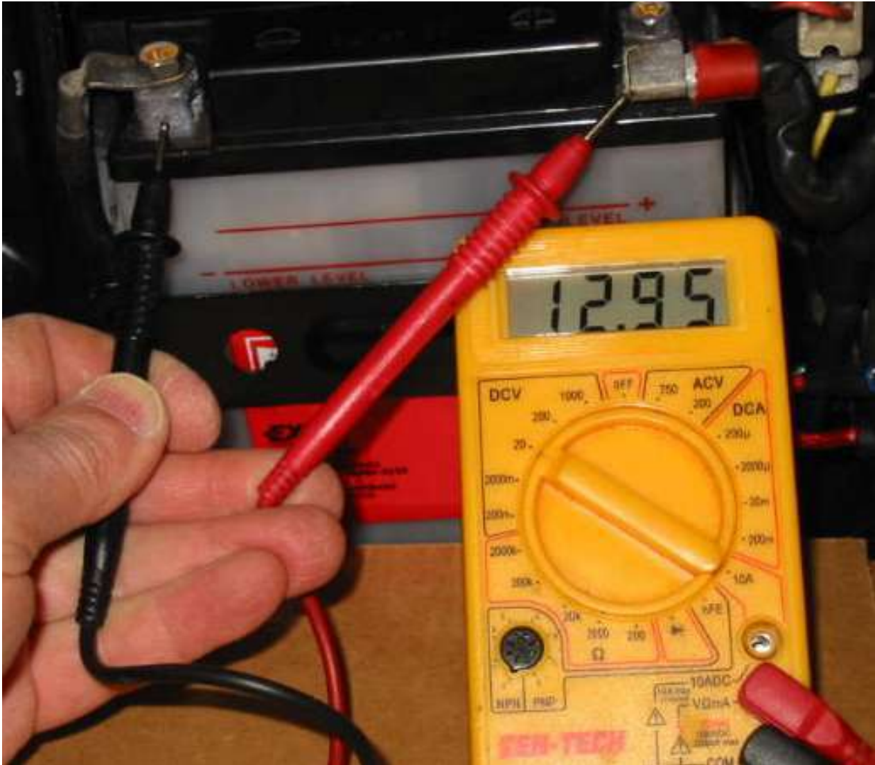
Figure 147: Battery Load test using Multimeter
