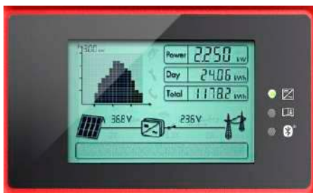
Figure 79: LED Green - Indicating correct operation of inverter
