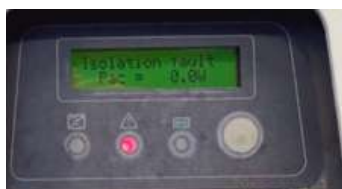
Figure 80: LED Red - Indicating incorrect operation of inverter
