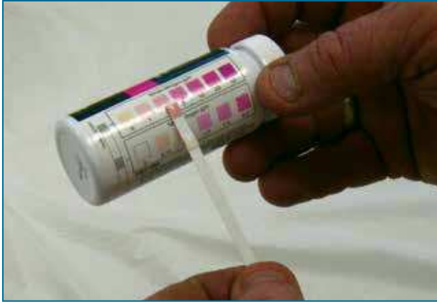
FIGURE 50. Home water-testing kits typically rely on a color change on a test strip to determine the concentration of a contaminant.
