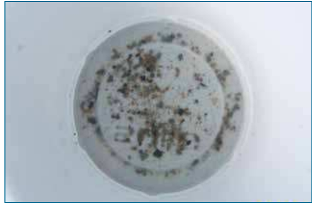
FIGURE 36. Sand accumulated on the screen of an irrigation system. (Source: Mike Prestigiacomio)
