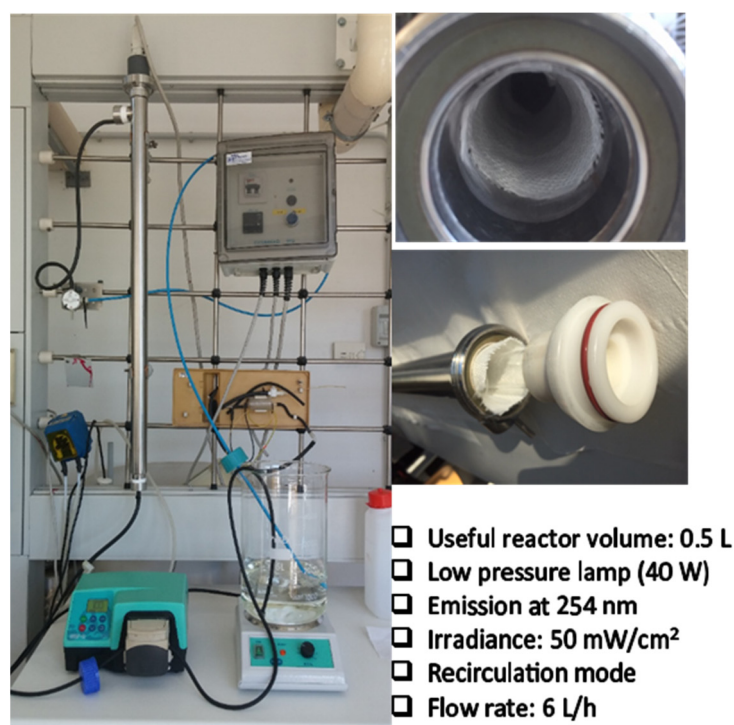
Figure 5. Photocatalytic system equipped with UV lamp, quartz tube and mesoporous titanium dioxide supported on glass fiber mats.
