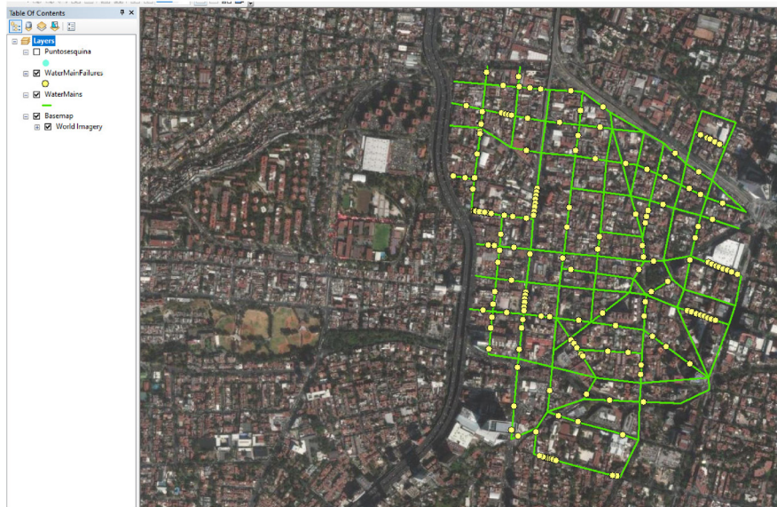
Figure 14.34 Water main grid with water main failures.
