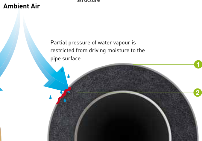
Figure 5. Materials with closed cell structure offer built in defence against water and water vapour ingress.
