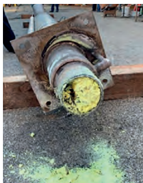
Figure 1. View of solidified sulfur in an extracted sulfur leg (left), and sulfur cake accumulated at the base of a sulfur pit that went 'cold' during a unit-wide power outage (right). Note the extensive damage to the sulfur pit walls due to sulfurous acidic attack exposing embedded steel bars (for reinforcement).
