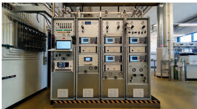
Figure 1. Servomex's Multigas Analytical System consists of four 19 in. racks including the SERVOPRO Chroma, MonoExact DF310E and DF745SGMax.
