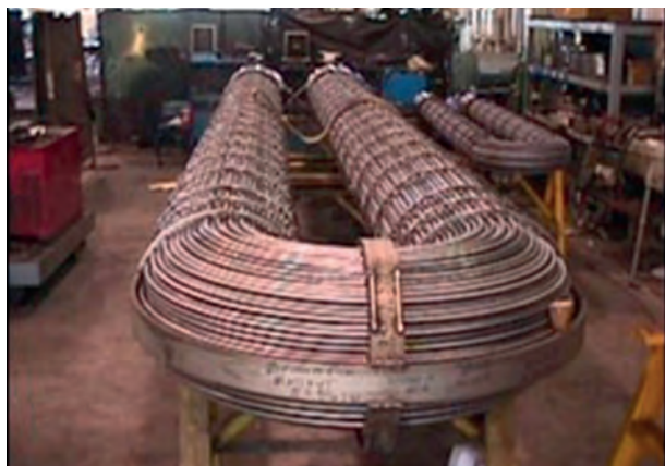
Figure 4. Hairpin bundle with large radius U-bends.
