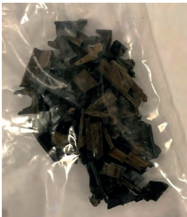
Figure 5. Cooling tower fill observed in the heat exchanger.
