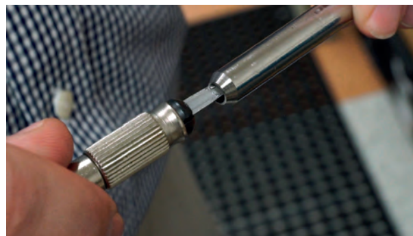
Figure 4. Traditional cone and thread fittings are not designed for ease of installation.
