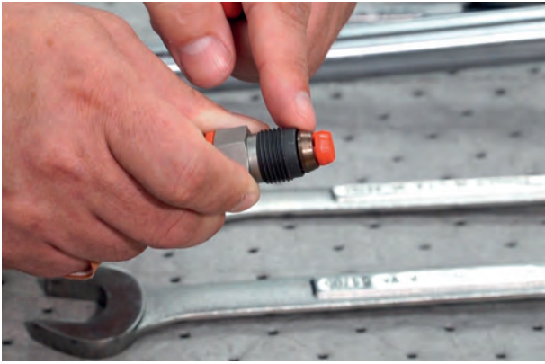
Figure 6. Fittings with pre-assembled cartridges can reduce installation times by 80%.
