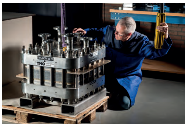
Figure 2. A PEM electrolyser R&D short stack developed by TNO and Hydron, to be used to test novel components on an industrial-scale (source: TNO).
