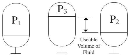
The precharge pressure is chosen to 90% of the min. working pressure.  $n$  varies between 1 and 1.4 depending on whether the charge is slow (isothermal) or fast (adiabatic).
