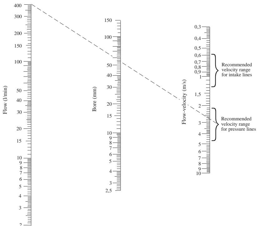
Nomogram for determining pipe sizes in relation to flow rates and recommended velocity ranges.
