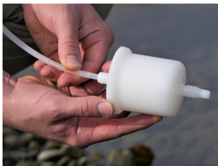
VOC tubing inserted into an eDNA filter.
