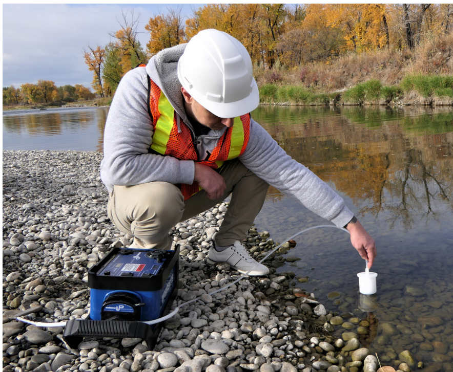
eDNA sampling using a peristaltic pump and eDNA filter.
