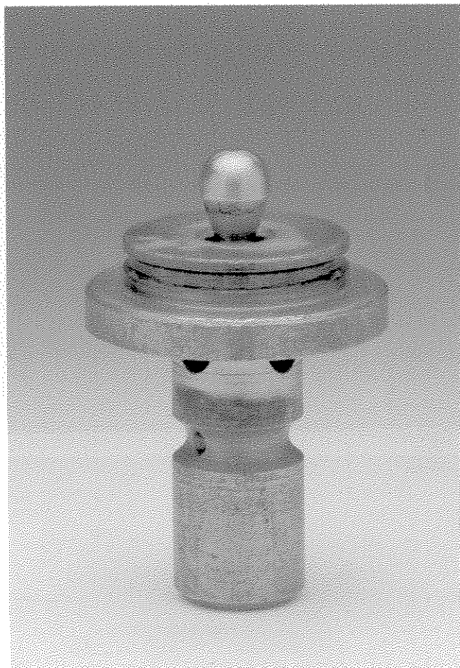
Fig. 241: Normal wear of the cone of a direct-operated pressure relief valve operating very frequently and after a long service life
