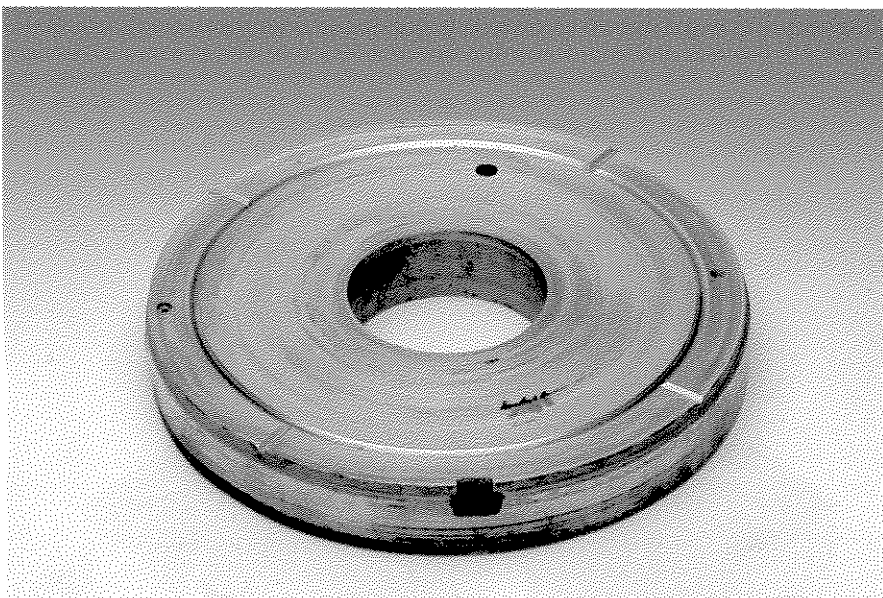
Fig. 245: Cavitation damage to the end cover of a vane pump caused by insufficient pressure at the pump inlet
