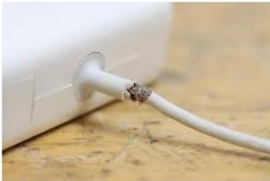
Damaged cable insulation
