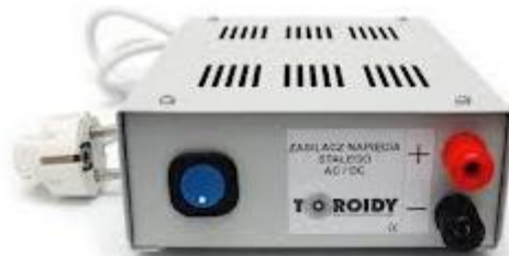
Rectifier (Device that converts AC to DC)
