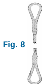
Fig. 8 HAND SPLICED SOFT EYE
