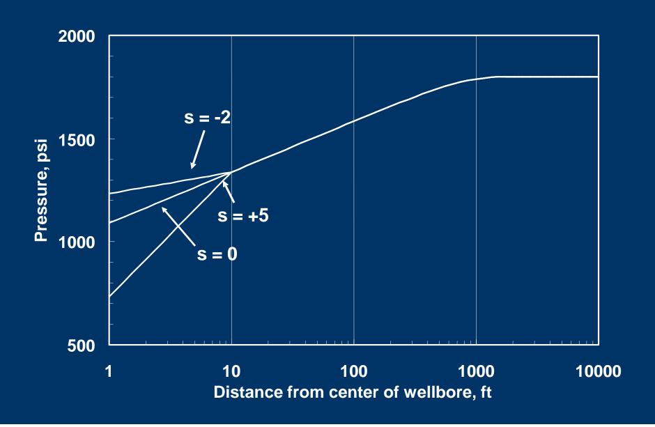
So ==> Skin is <u>CHANGE IN PRESSURE DROP</u> that exists near the wellbore in "real wells" compared to a "Darcy-model" of the well
