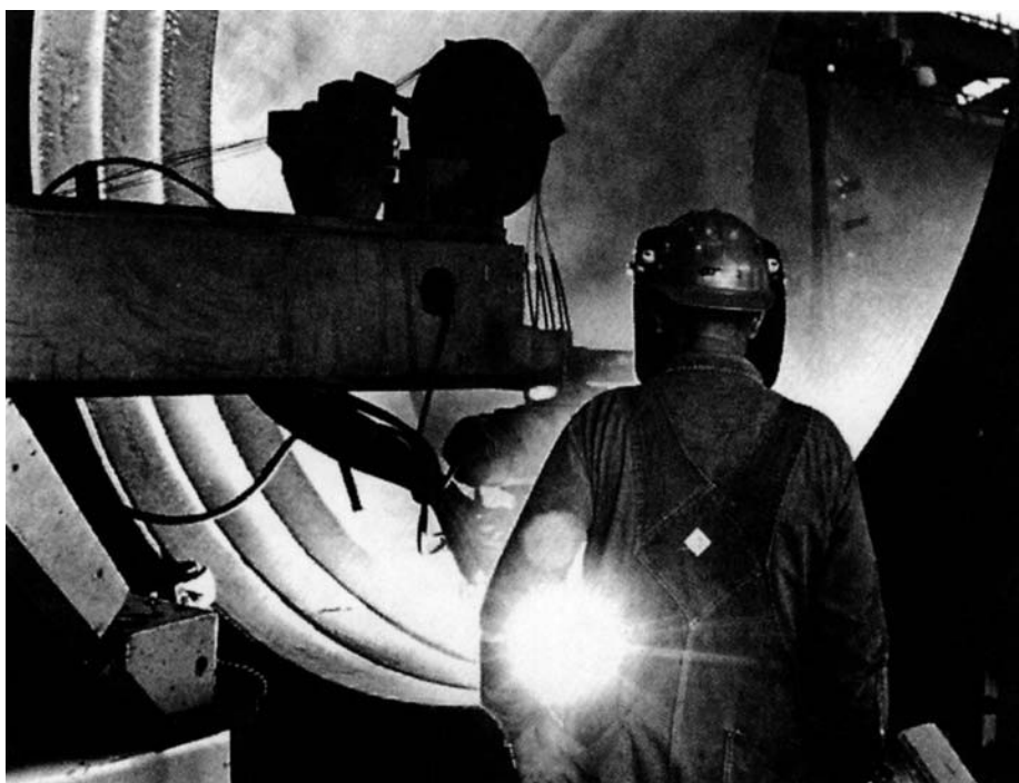
Process reactors in a petroleum refinery can either be solid stainless steel (above), clad, or protected with a weld overlay (below), such as might be used in an HDS reactor.
