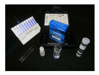
Figure 8.4. Peroxyacetic acid concentration can be measured with a colormetric test kit or test strips.
