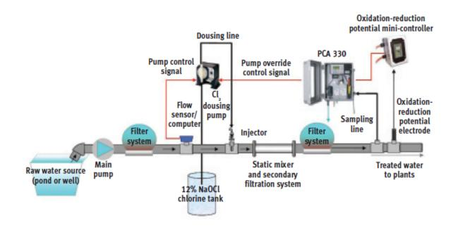
Figure 5.2. System diagram to inject and control liquid chlorine (sodium hypochlorite).
