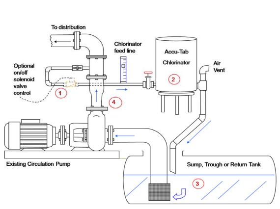
Figure 5.4. System diagram for calcium hypochlorite.
