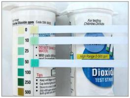
Figure 7.4. Chlorine dioxide concentration can be measured with a meter or test strips. Photograph by Peter Konjoian.
