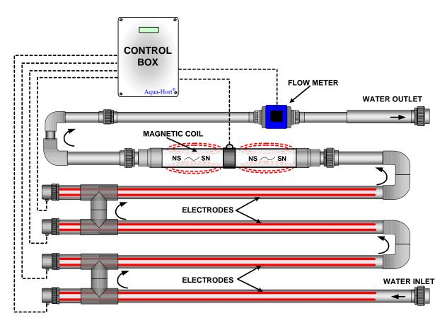
Figure 9.1. This AquaHort copper system is equipped with copper electrodes inside pipes. An electrical current passes through the system to turn solid copper metal electrodes into soluble copper ions. A magnetic coil increases activity of the copper ions. The control box corrects ionization rate based on water flow and water electrical conductivity to maintain a constant copper concentration.
