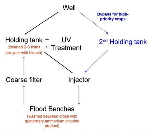
Figure 12.2. Two water circulation patterns from a tropical plant propagator. The existing flow pattern (shown in black) mixed fresh well water and return water in the holding tank. A new tank (blue) was added for crops that only received clean well water.
