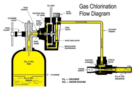
Figure 6.1. A gas chlorination flow diagram. Image courtesy of Chlorinators Incorporated.
