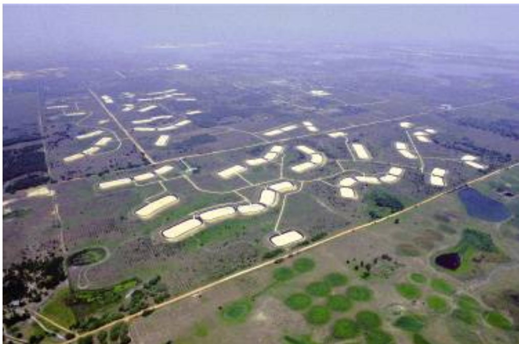
FIGURE 2-14 Rapid infiltration basins at the Water CONSERV II facility in Orlando, Florida, which recharged 31 MGD (120,000 m 3 /d) of reclaimed water in 2006.
