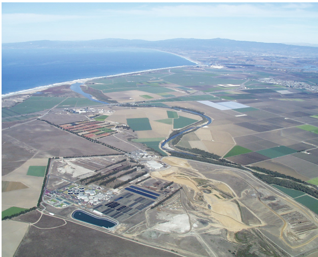
FIGURE 2-9 The Salinas Valley Reclamation Project in Monterey, California, which provides reclaimed water to area farms, thereby reducing seawater intrusion caused by overpumping the region's aquifers. SOURCE: Monterey Regional Water Pollution Control Agency.
