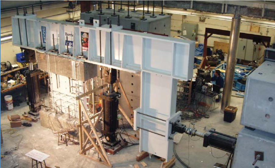
Wallace's team performs a test of both horizontal and vertical loads on a reinforced concrete wall panel.
