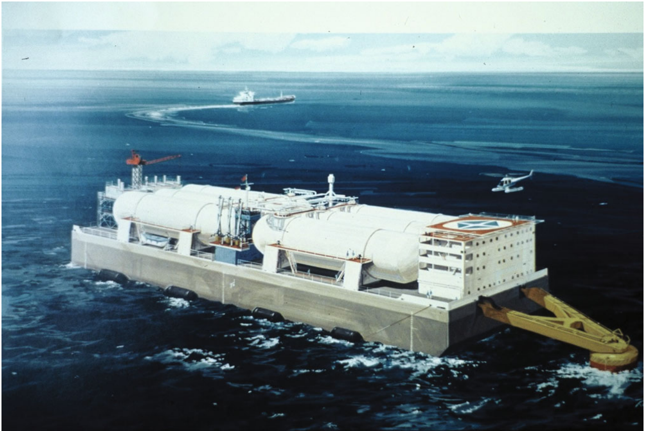
Fig. 4.6 “Artist view”, Arco Barge. The barge, or rather, the LNG gas terminal, was designed and built in concrete in a dock in Tacoma, Washington, USA in 1973. For the construction 25 000 tons of concrete was used. Length 140.5, 41.5 m, depth 17.2 m. After birthing,
