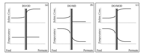
Fig. 5. Concentration and temperature profiles in (a) DO/OD, (b) DO/MD, and (c) DO/MOD.
