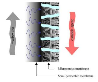
Fig. 2. Mass transport in the dual DO/OD membrane process in DOC#2.
