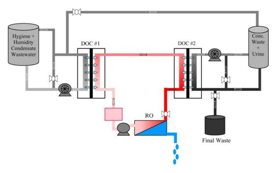
Fig. 1. Flow diagram of the NASA DOC wastewater treatment process.
