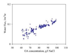
Fig. 3. Flux vs. OA concentration in the dual DO/OD process.
