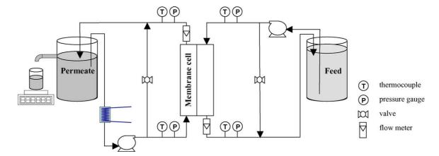
Fig. 6. Flow diagram of the bench-scale test unit.
