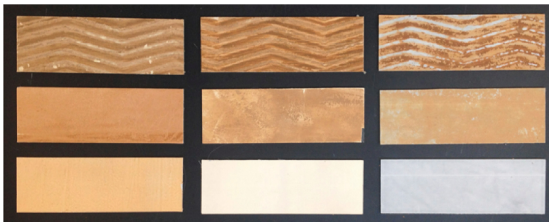
Fig. 3. Images of virgin and fouled CTA, TFC1, and TFC2 membrane samples. Fouled coupons are from membranes used under test set A and test set B conditions.
