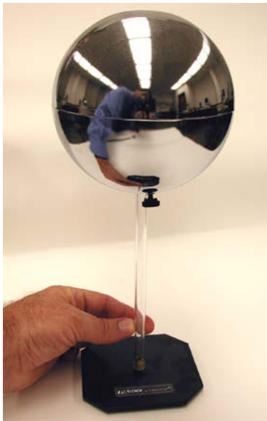
Figure 9-10. Conducting sphere, supported by an insulating base. When you move the sphere, touch the base, not the sphere, to avoid disturbing its charge.
