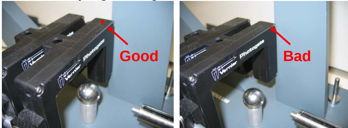
Figure 6-7. Using the ball carrier to adjust the height of the photogates.
