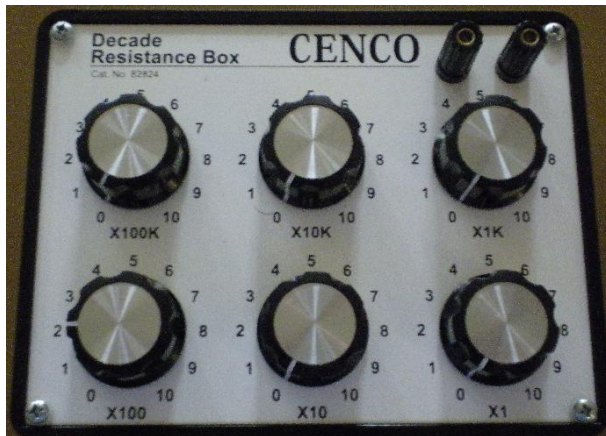
Figure 11-12. Adjust the decade box for 200 \Omega as shown here.
