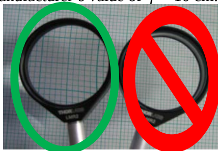
Figure 13.7 Use the converging lens, not the diverging lens, for Part I.
