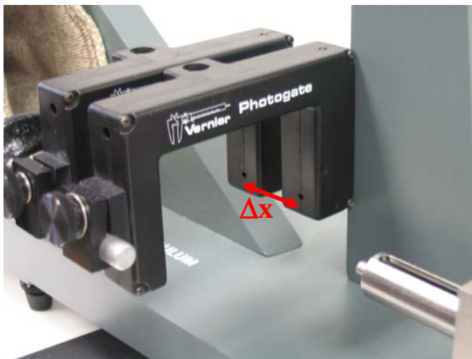
Figure 6-6. Alignment and positioning of photogates. They are similarly aligned and the tops touch.
