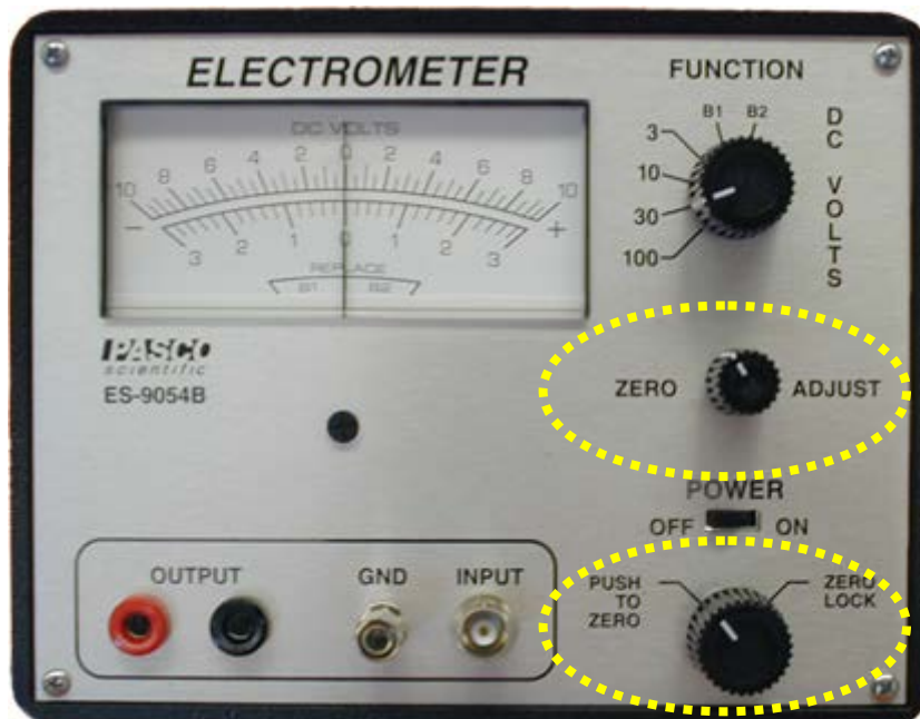
Figure 9-7. To zero the electrometer, hold down the “PUSH TO ZERO” button while turning the “ZERO ADJUST” knob, until the needle points to 0. Use the top scale for reading using the “10” or “100” scales (multiply your reading by 10 if on the “100” scale) and the bottom scale for the “3” or “30” scales (multiply your reading by 10 if on the “30” scale).
