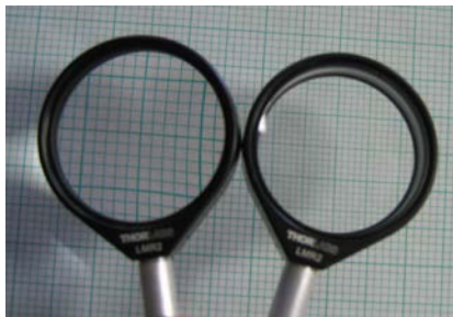
Figure 13.3. “Object” and “image.” Here, the sheet of graph paper is the “object”. What you see through the lens is the “image.”
