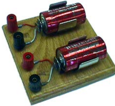
Figure 11-2. Board with two batteries.
