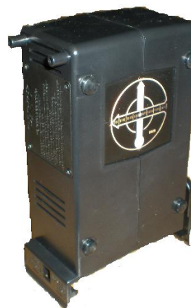
Figure 13.4. An “object” you will use is this back-lit cross. The backlighting itself isn’t of interest; it merely helps provide good contrast so that you can easily see the cross. There’s an arrow on the cross so that you can tell whether an image of it is inverted.
