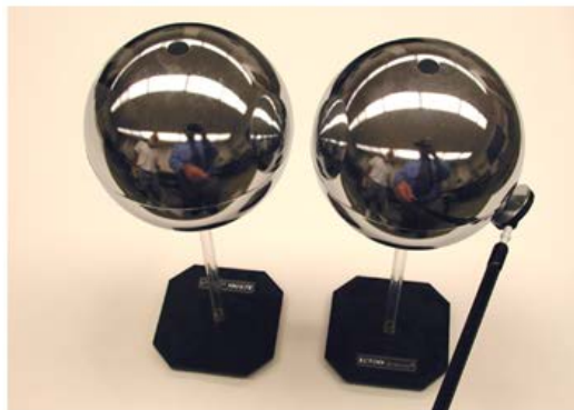
Figure 9-13. Procedure for Part B, with two spheres. Be sure that the charged insulator is held in place while separating the two spheres in step 5.
