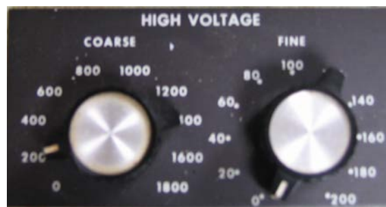
Figure 16-3. Set the High Voltage on the Control Unit to a value equal to 50-75 volts above the threshold value given to you by the TA. Do not exceed the maximum voltage indicated by the label on the top of the control unit.
