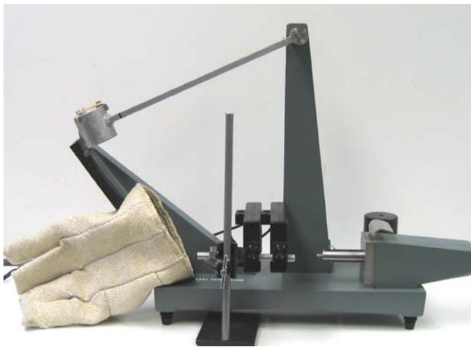
Figure 6-5. Setup for Part II. Note that the pendulum bob is up on the rack and that the glove is propped open ready to catch the ball after it goes through the photogates.
