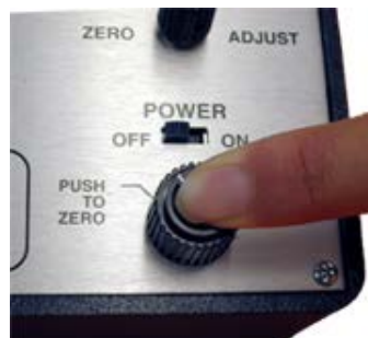
Figure 9-9. The other method to ground the Faraday ice pail: press the “PUSH TO ZERO” button on the electrometer.
