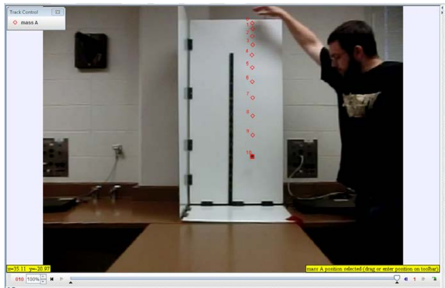
Figure 3-3. Screen shot of the last frame of a movie. Note the track showing the position of the ball in each frame.
