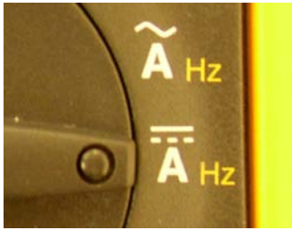
Figure 11-10. Adjust the multimeter for a 20 mA scale. Be sure to select DC, not AC current. (Your meter may look different.)
