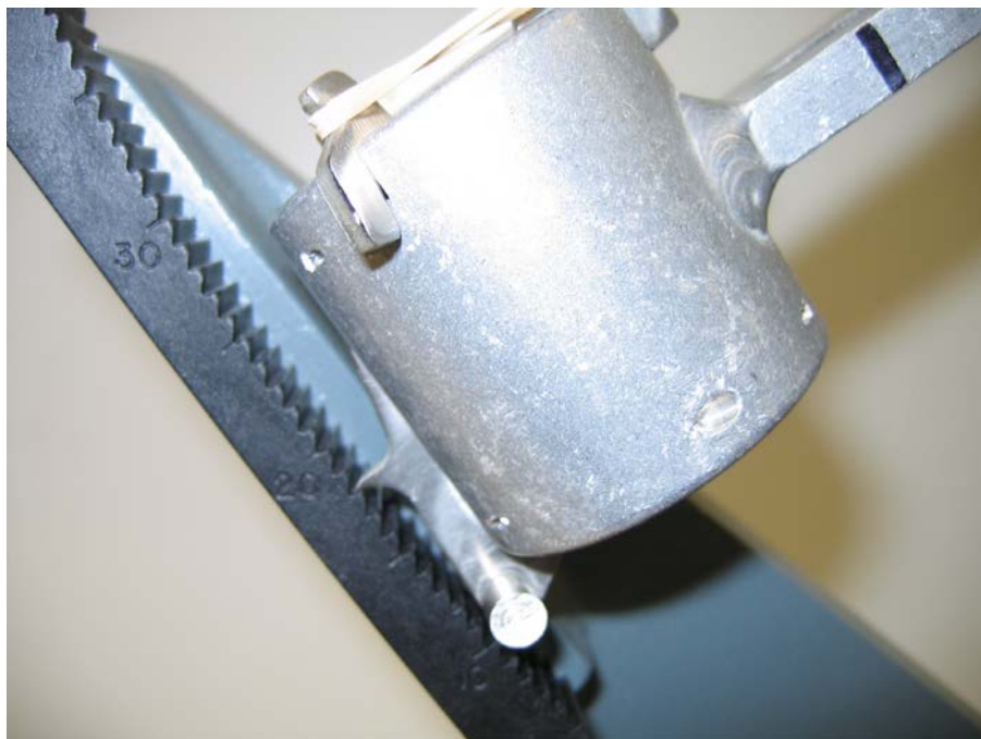
Figure 6-9. Pendulum bob caught by rack after the ballistic pendulum is fired. In this picture the pawl is caught in notch #18.
