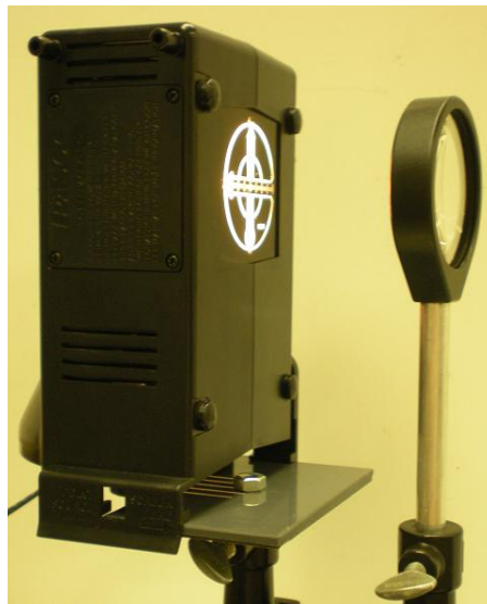
Figure 13.11. Adjust the object box and lens to the same height.
