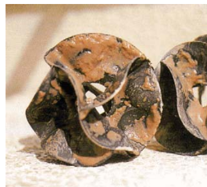
Figure 2.- Typologies of plastic support used as filling media for trickling filters
