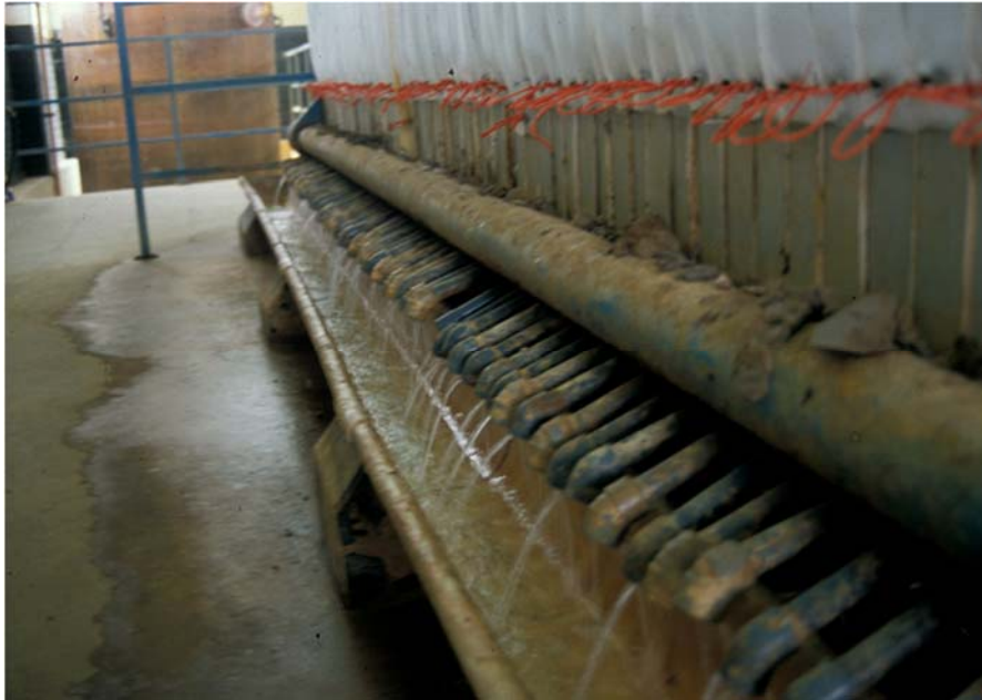
Figure 24. Filtered water after each filter cell in a press filter.
