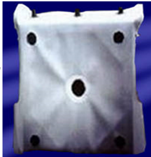
Figure 8.- Press filter cells scheme and filtering cloth arrangement view.
