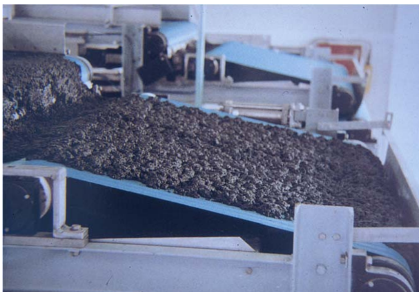
Figure 15. Sludge over filtering cloth on a band filter prior to entering compression stage.
