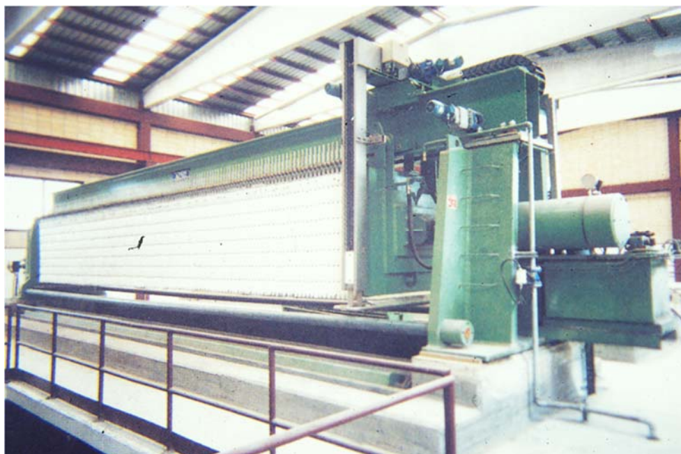
Figure 21. General view of a press filter.
