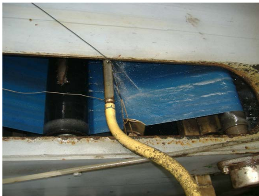
Figure 17. Band filter cloth washing by ejectors.
