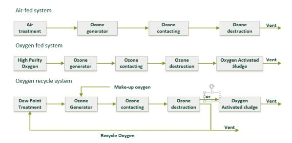
Figure 4 Diagram with different ozonizator feed options (mod. from US EPA, 1986).
