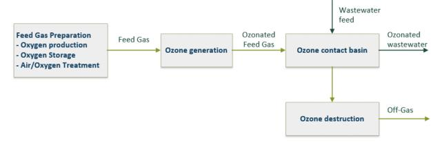
Figure 2. Simplified ozone process schematic diagram (mod. From US EPA, 1986)
