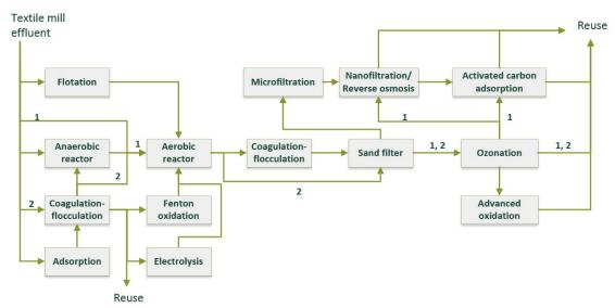
1: High Lura WWTP managed by CIDA Srl in the area of Como (Italy) treating 22,000 m³/d of a mixture consisting of 17% domestic WW, 32% rainwater, 51% textile finishing mill equalized effluent (cellulose, wool, silk and synthetic fibers. 2: Levi's Strauss WWTP, Wervik (Belgium).
