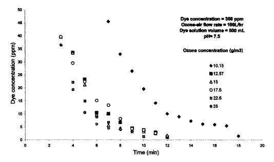
Figure 8.- Time vs concentration data at different ozone concentrations in a direct dye treatment (Konsowa, 2003).
