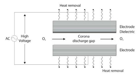
Figure 5.- Principal elements of a corona discharge ozone generator (mod. from US EPA, 1986).
