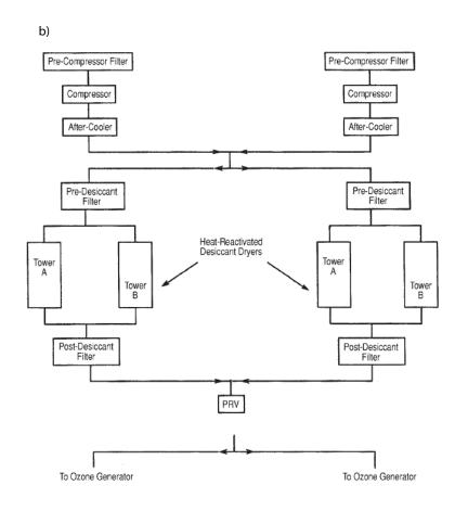
Figure 3.- Schematic diagrams for low (a) and high (b) pressure air feed gas treatment system (US EPA, 1986).
