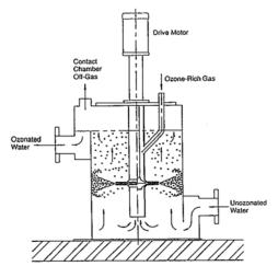
Figure 7. Turbine mixer ozone contactor (EPA, 1999)
