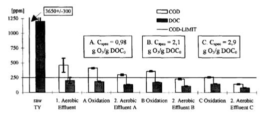
Figure 12.- Effluent quality parameters in successive stages with combined biological + ozone treatment to tannery effluent (Jochimsen, 1997).
