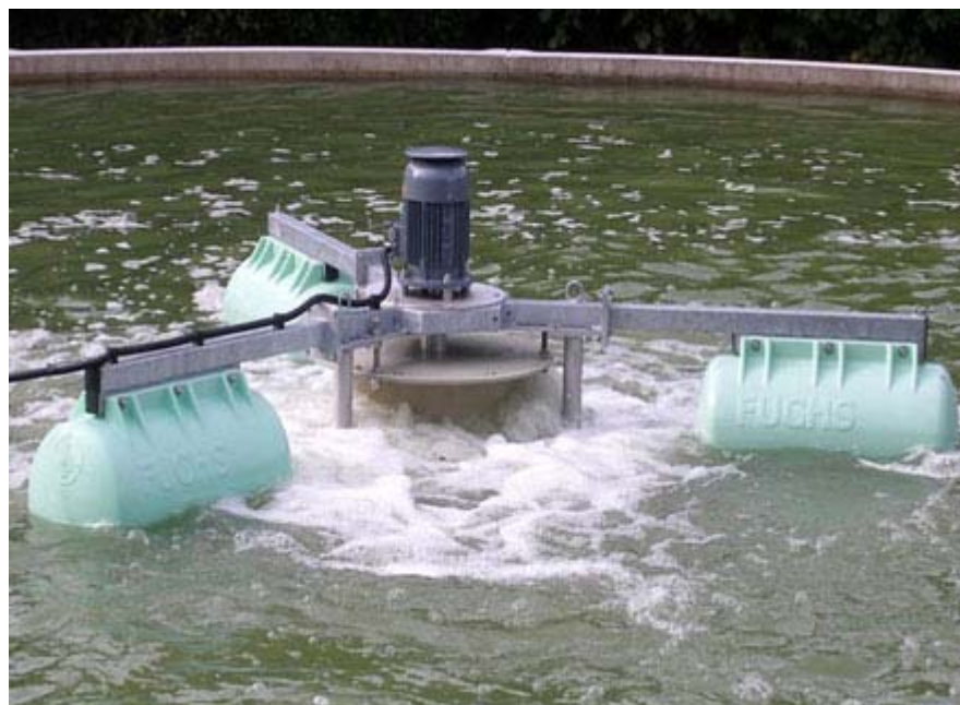
Figure 6 Vertical axis floating agitation/aeration system
