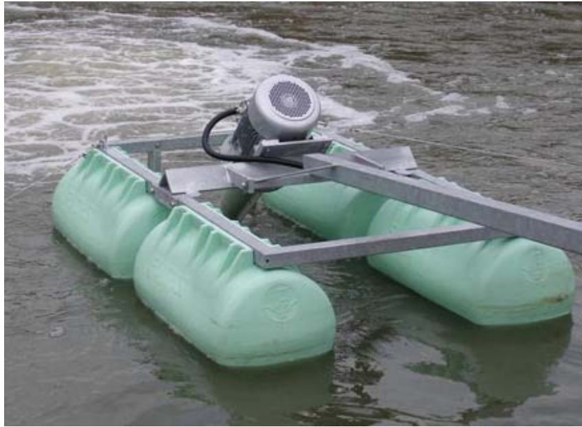
Figure 7 Oblique axis floating agitation/aeration system
