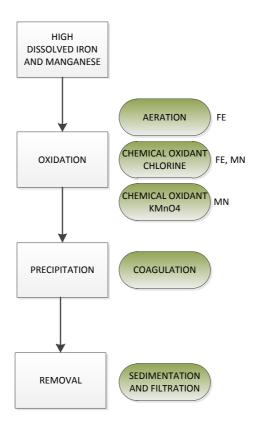
Figure 5-2: Treatment processes for dissolved iron and manganese in groundwater
