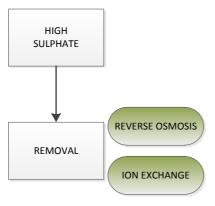
Figure 5-7: Treatment processes for sulfate
