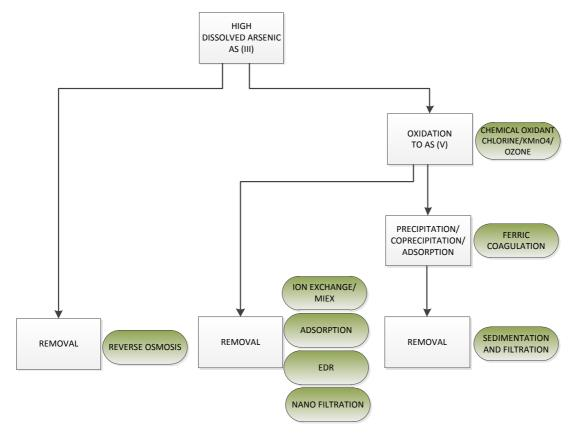
Figure 5-1: Treatment processes for removal of dissolved arsenic in groundwater
