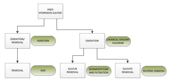
Figure 5-6: Treatment processes for hydrogen sulfide
