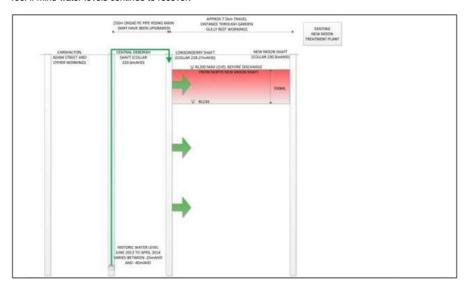
Figure 2-2: Current Dewatering Operations Schematic
