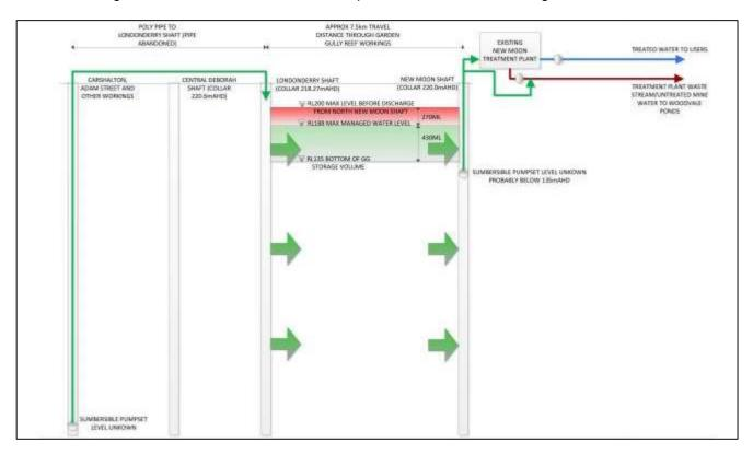
Figure 2-1: Historic Dewatering Operations Schematic
