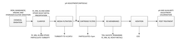
Figure 5-10: Schematic of New Moon Water Treatment Plant process, including waste streams
