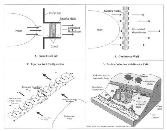
Figure 5-9: example configurations of PRBs (ITRC, 2005)
