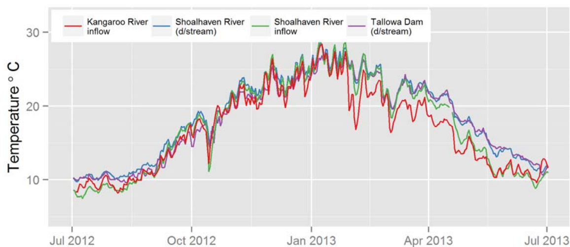
Figure 6.12 Shoalhaven system temperature profile
