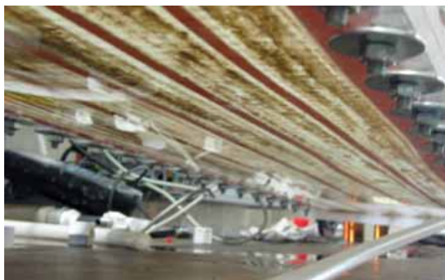
Figure 3.8 Photograph showing the feed side of the inverted forward osmosis membrane cell after three days of operation with no cleaning (The feed channel of the membrane cell is under the membrane)
