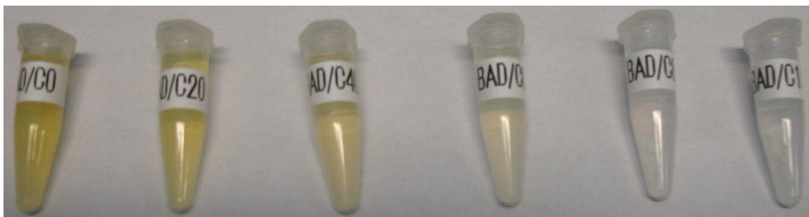
Figure 16: Sample B photocatalyst dye degradation.
