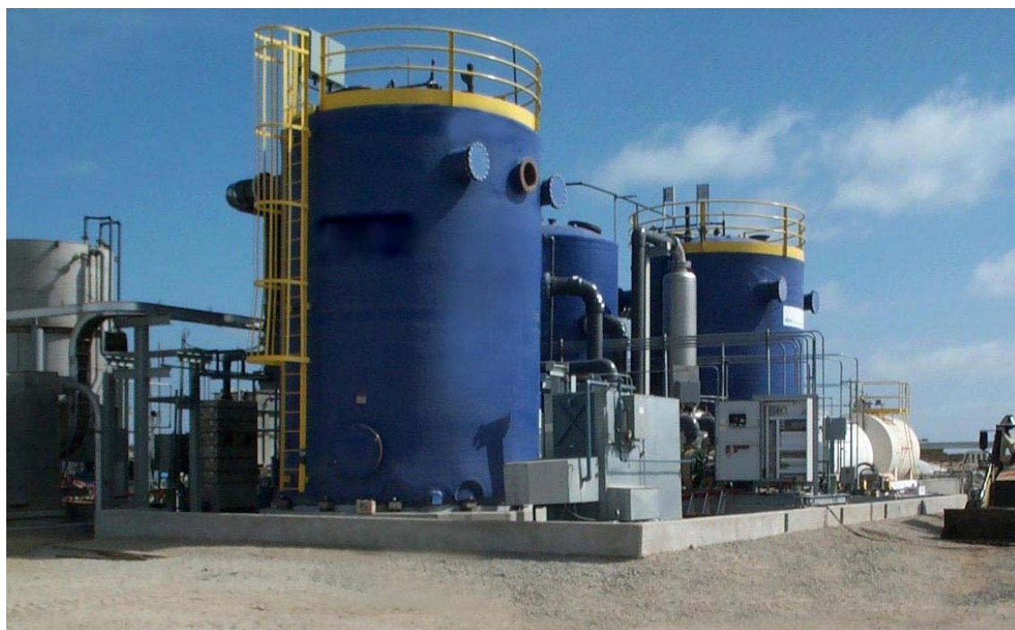
Figure 5 Fluidized bed reactors for treatment of industrial and urban wastewater (Envirogen system Technologies).
