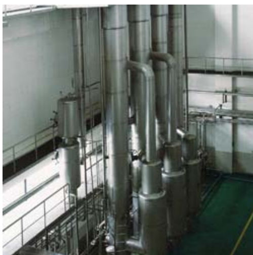
Figure 8.- Falling film evaporator JINZHOU GROUP CO., LTD. http://www.jzmachinery.com/IndustrialEvaporator.html (September 2015)
