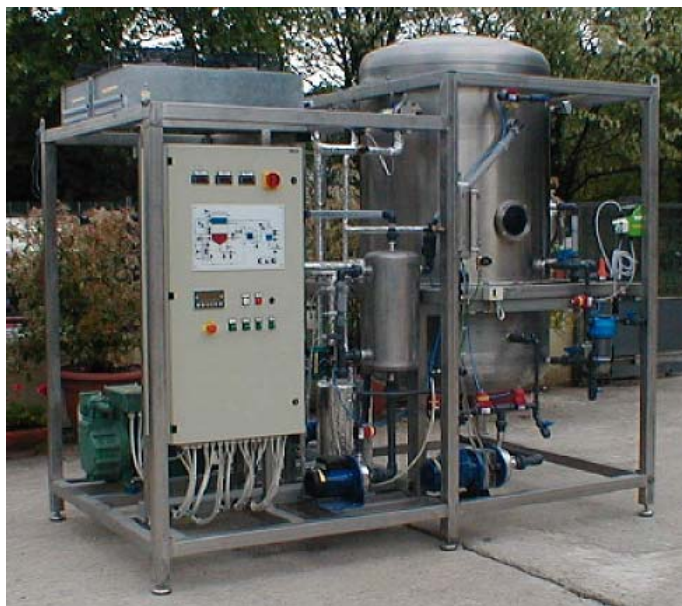
Figure 5.- VNT industrial vertical evaporator for printing line process effluent treatment. 90% of the water is recovered.
