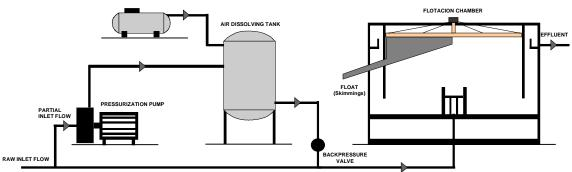
Figure 3.- DAF with partial inflow pressurization (CEPIS, 1992.
