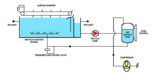
Figure 11.- Rectangular flotation tank scheme.
