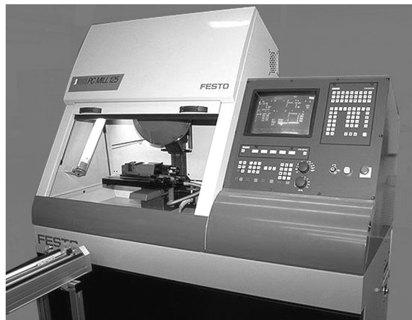
Automatic door of the CNC machining centre
