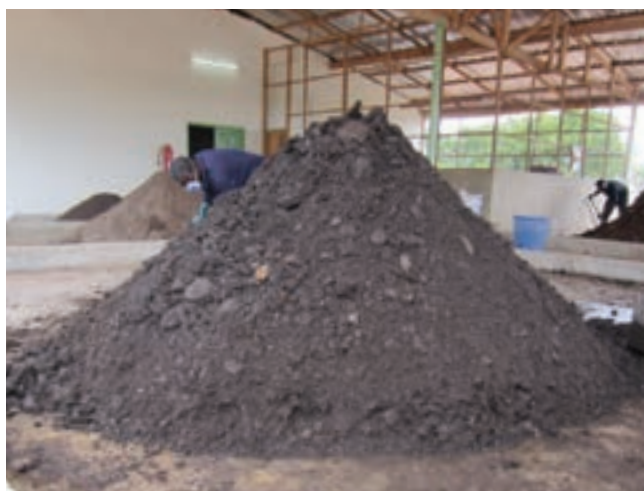
FIGURE 16. HEAP COMPOSTING OF DEWATERED FS.
