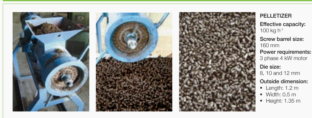
FIGURE 23. PELLET PRODUCTION – A) PELLETIZER BEING OPERATED, B) NEWLY PRODUCED PELLETS, AND C) FINAL PELLETS (AFTER DRYING AND SIEVING).
