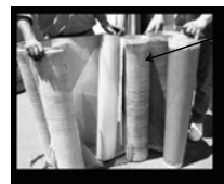
A membrane severely fouled by organics
