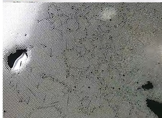
Recrystallisation Defected bubble raft analogous to cold working metals
