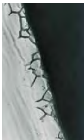
Intergranular corrosion of stainless steel
