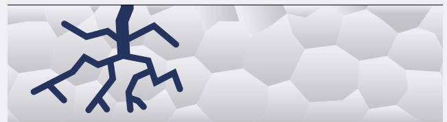
Fig. 1.6.10: Stress corrosion cracking
