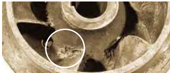
Cavitation corrosion of bronze impeller
