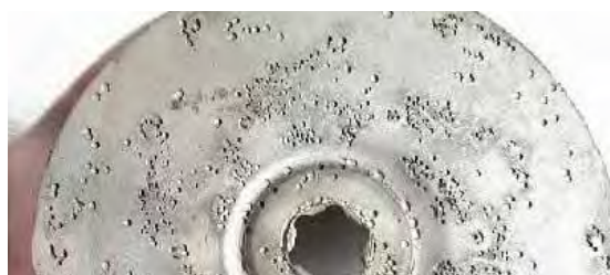
Pitting corrosion of EN 1.4401 (AISI 316)
