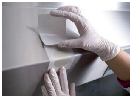
Figure 1. Examples of direct contact and swab sampling using 3M™ Petrifilm™ Plates
