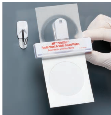
Figure 2: Example of air sampling using 3M™ Petrifilm™ Plates
