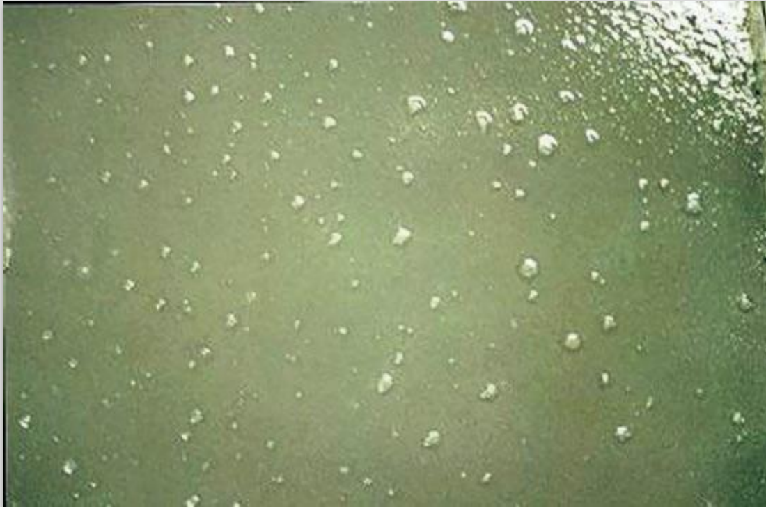
Fig. 38 Solvent (clear) bubbles on the surface of the paint film soon after application.
