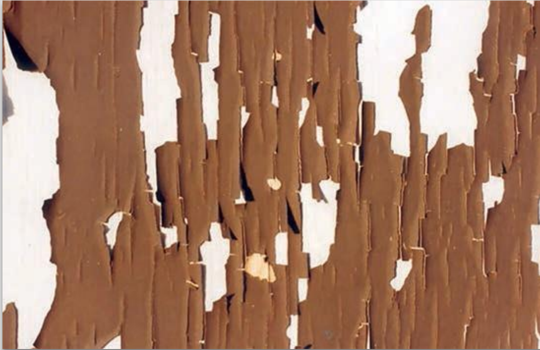
Fig. 20 A form of adhesion failure where paint flakes from the substrate. A familiar sight on wood substrates and on galvanizing.
