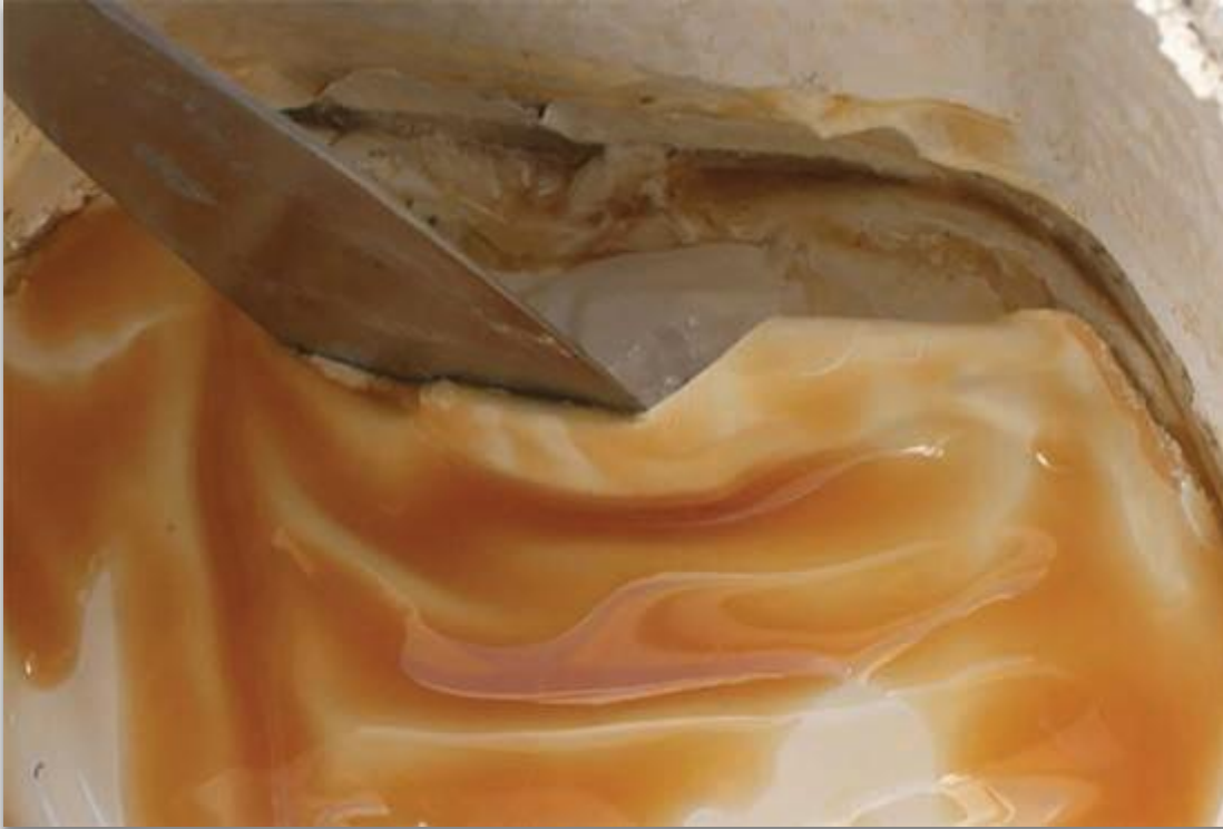
Fig. 36 Formation of a layer of skin on the paint surface in a container.
