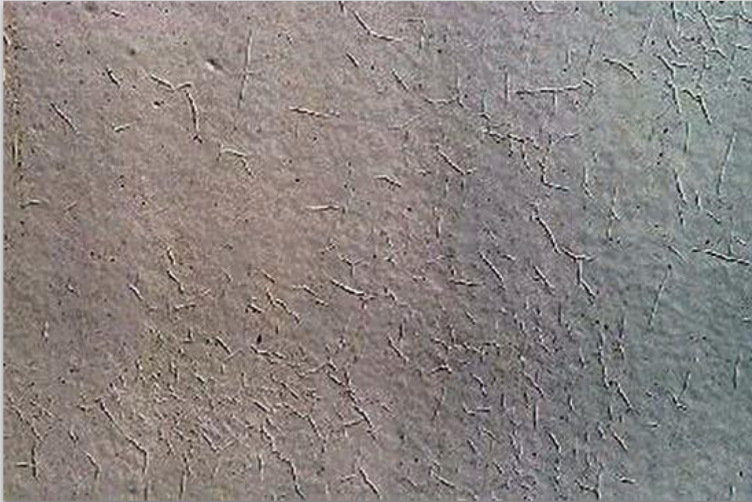
Fig. 17 The development of small wrinkles in the paint film in a pattern resembling a crow's foot.
