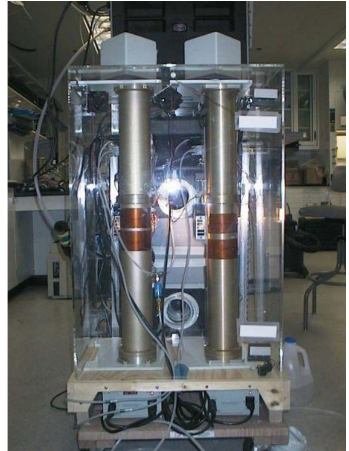
A nephelometer at the Kosan, Cheju Island, South Korea NOAA facility.
