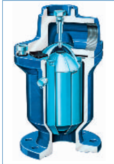
Fig. 8.2-a: Duojet*) two-way air valve with a medium-operated single-compartment valve.
