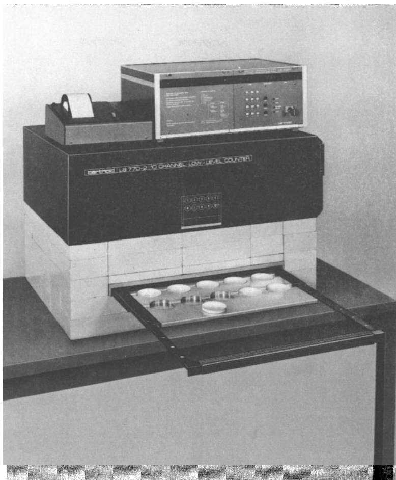
Fig. 116. Low-level measuring station for simultaneous measurement of 10 alpha or beta emitters in sample dishes with a diameter of 60 mm following chemical separation of individual nuclides or nuclide groups from water sample
