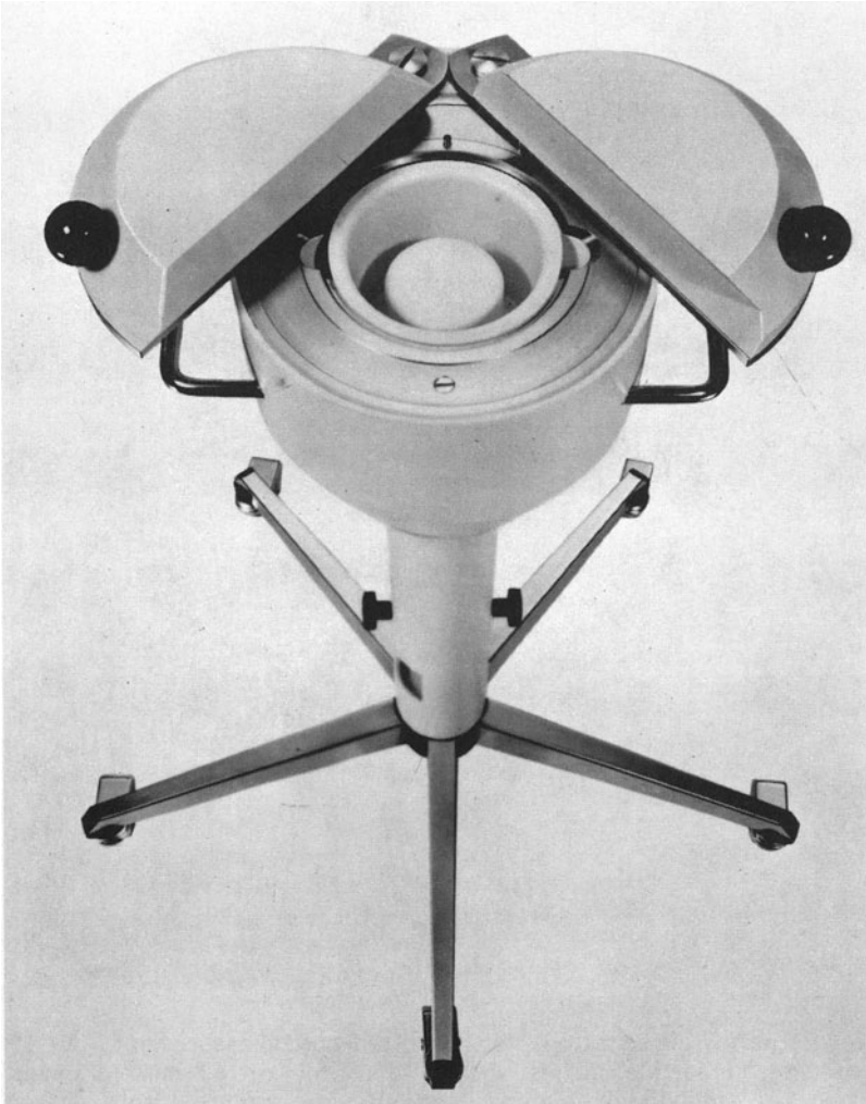
Fig. 117. Sodium iodide scintillation counter with ring-beaker arrangement for measurement of gamma emitters directly from the water sample
