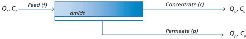
Figure 5 RO membrane mass balance schematic
