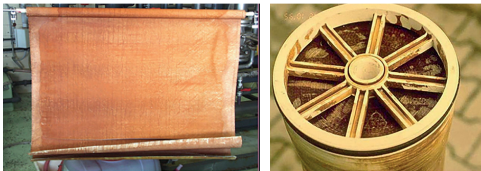
Figure 8 Membranes fouled with iron (left) and manganese (right) (DuPont, 2020)
