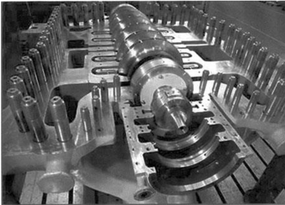
Interior of centrifugal compressor
