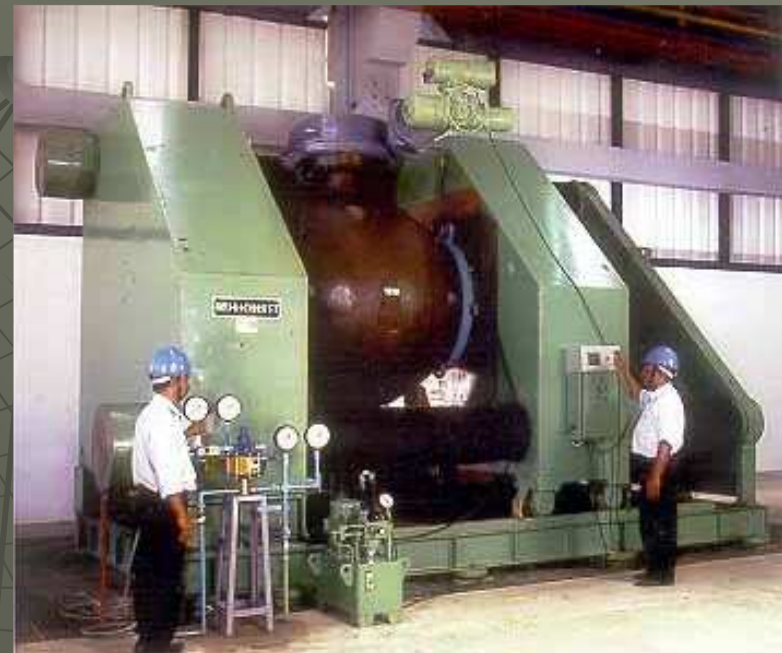
42" Trunnion-mounted Ball Valve undergoing Hydro test
