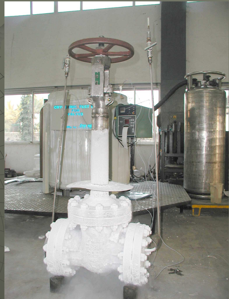
Valve after Cryogenic Test
