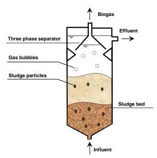
Figure 2.- Schematic drawing of a UASB reactor.
