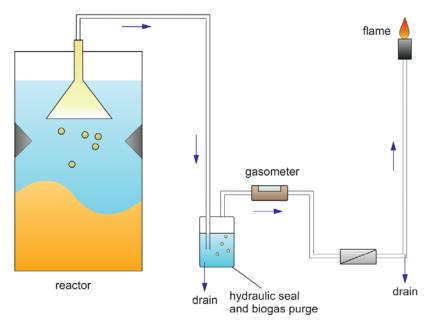
Figure 5.- Diagram of a gas system in UASB reactors with a hydric seal.
