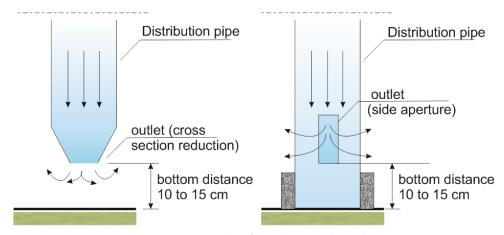
Figure 4.- Examples of distribution tube ends.
