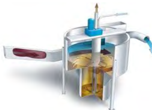
Figure 2-6 Screen and Compactor
