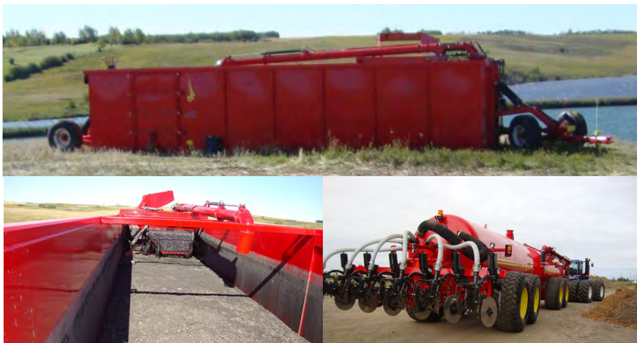
Figure 5-6 Frac Tank (top) Coarse Screen (bottom left), QuadVac (bottom right)
