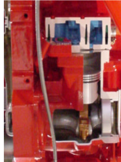
Air Compressor Cummins Diesel Engine
